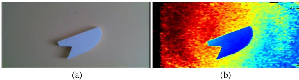
**Figure 2.** The image of camera D415, default setting: (a) RGB image and (b) depth image
