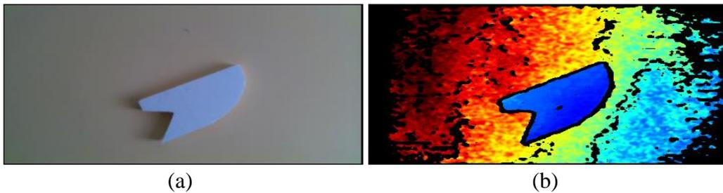
**Figure 4.** The image of camera D415, high-accuracy setting: (a) RGB image and (b) depth image
