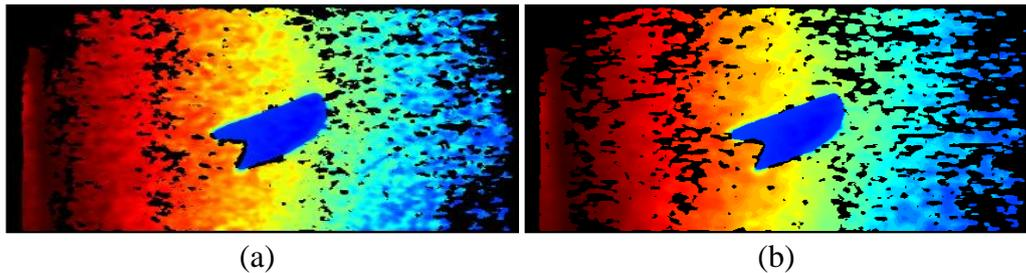
**Figure 7.** The image of camera D435, high-accuracy setting: (a) with factory-set filters for keeping the edges and (b) with random-set filters for keeping the edges
