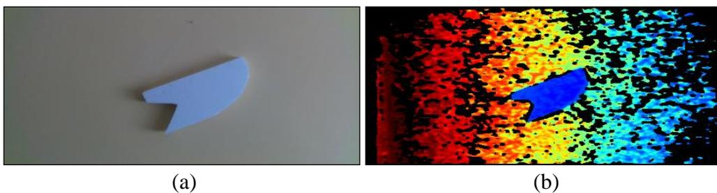
**Figure 5.** The image of camera D435, high-accuracy setting: (a) RGB image and (b) depth image
