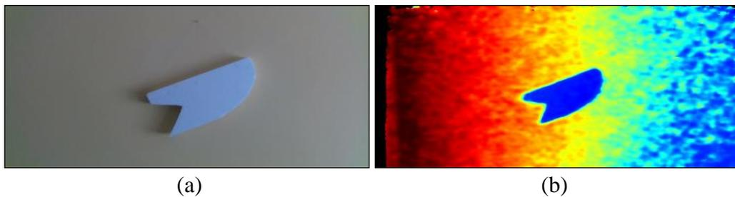
**Figure 3.** The image of camera D435, default setting: (a) RGB image and (b) depth image
