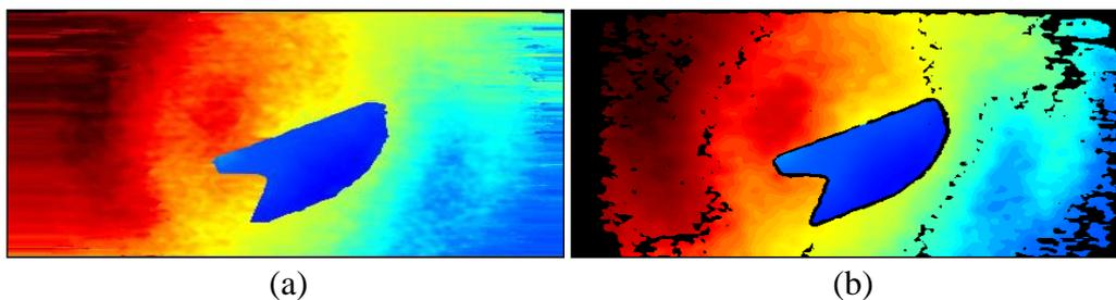
**Figure 6.** The image of camera D415, high-accuracy setting: (a) with factory-set filters for keeping the edges and (b) with random-set filters for keeping the edges
