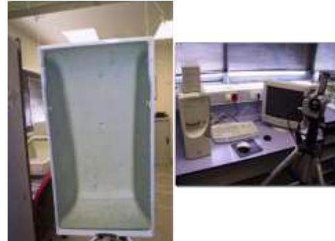
Figure 1: The image on the left shows the part analysed, a fibreglass radome. In the image on the right, the High Speed Thermal Imaging Equipment.
