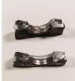
Figure 13: Top and bottom sections of the riveted sample
