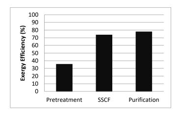
Figure 4. Exergy efficiency for the main stages
