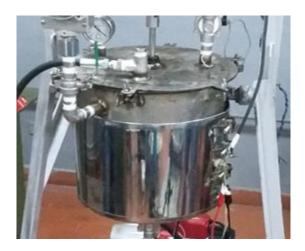
Figure 5. Osmodehydrator tank
