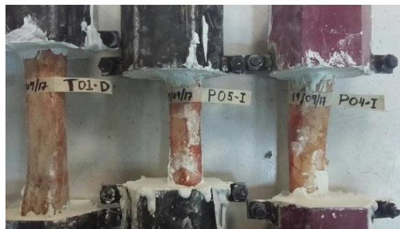
Figure 2. Test-tubes ready to perform the destructive test of flexion at 3 points.
