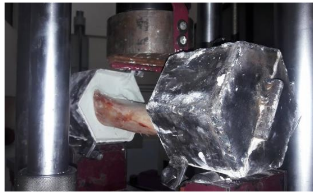
Figure 3. Assembly of the test piece in the test machine.
