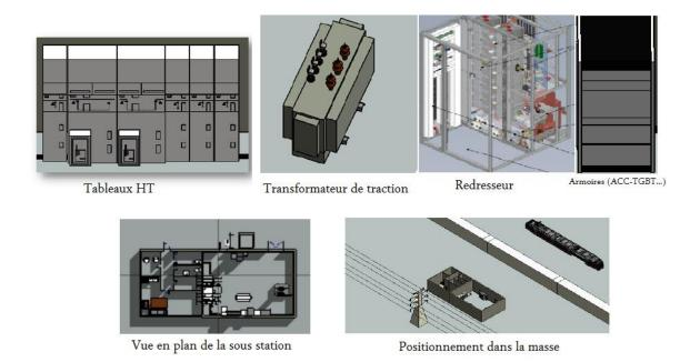
Fig.3: Model visualization of the Colas Rail/ONCF substation.
