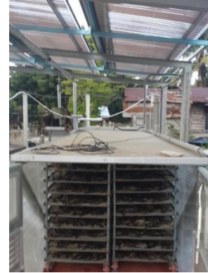
Fig. 3 Photograph of greenhouse solar dryer with heat exchanger
