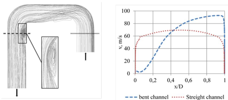
Fig.1: Flow in bent channel of steam supply system of steam turbine
