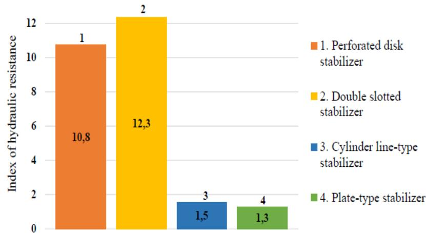
Fig.3: Comparison of flow stabilizers by hydraulic-resistance index
