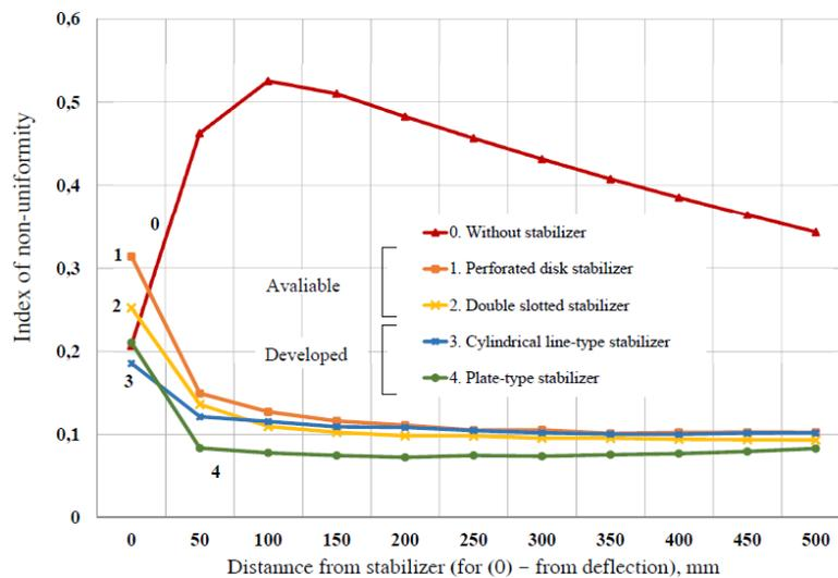
Fig. 2: Comparison of flow stabilizers by non-uniformity index
