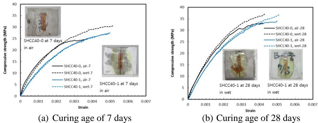
Figure 3. Typical compressive behaviors of PVA-SHCC mixtures
