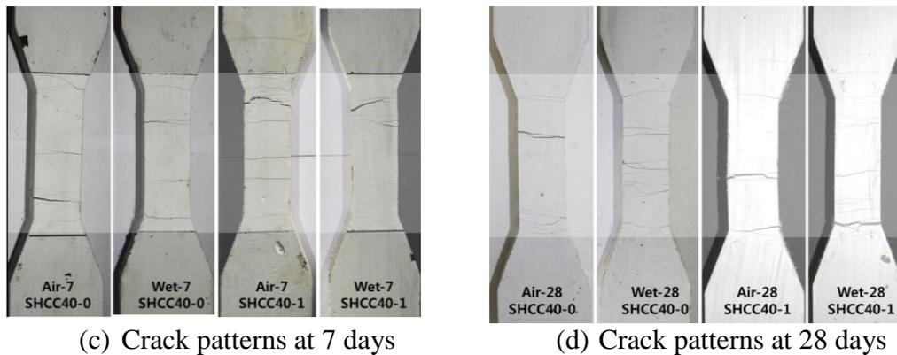
Figure 5. Typical tensile behaviors and failure modes of PVA-SHCC mixtures
