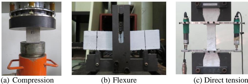
Figure 2. Testing rig for evaluating compressive, flexural and tensile performance
