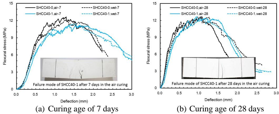
Figure 4. Typical flexural behaviors of PVA-SHCC mixtures
