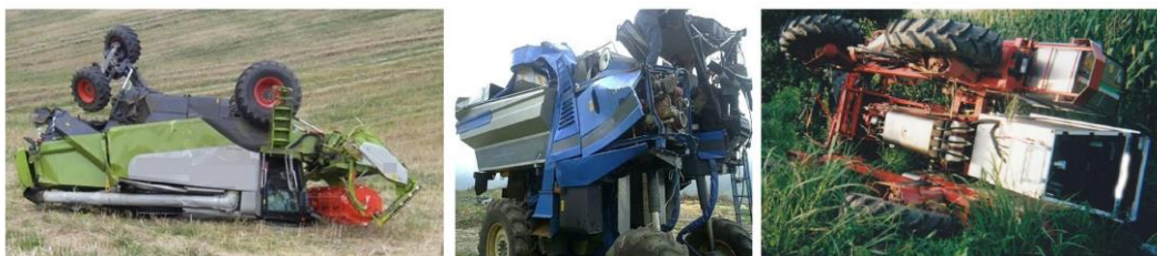
Fig. 1: The Self-Propelled agricultural Machinery are at risk of rolling over (courtesy of INAIL – Rome, Italy)
