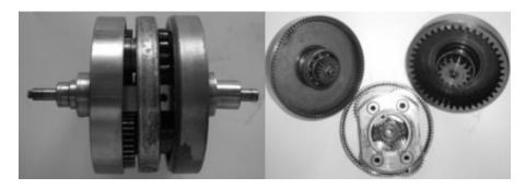
Figure 1: The design of the planetary system of universal multi-threaded differential mechanism
