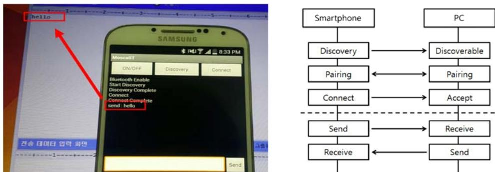
Fig. 2. Test App and Communication flow
