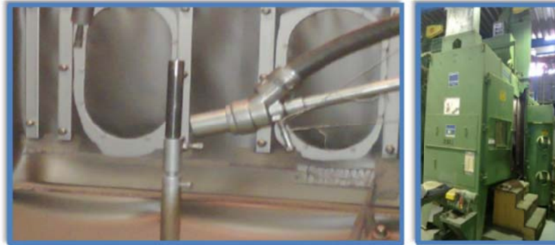
Fig .4 A : Inside view for shot peening machine and holding base B) : Shot peening machine.
