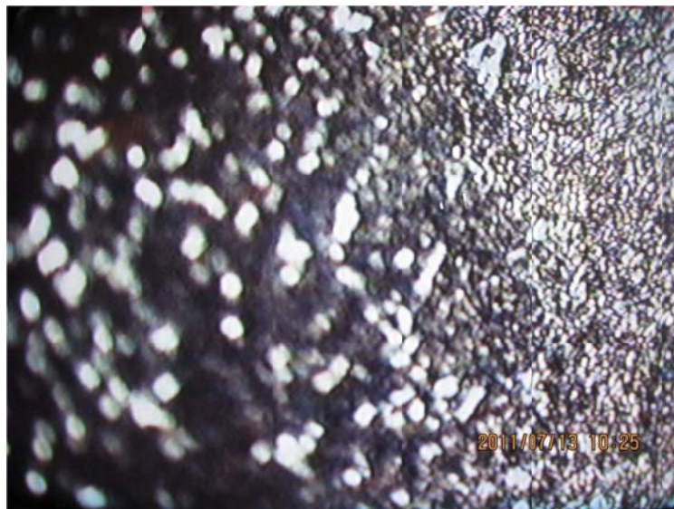
Fig.10 A micrograph of the surface deformation of the d2 heat treated alloy steel with magnification 200X (diamond pressing parameters for the specimen were: Pf=50 N Fp=0.12mm/rev).
