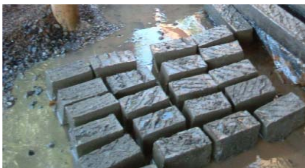
Figure 2 rough substrate surface prepared using grooving tool at fresh
