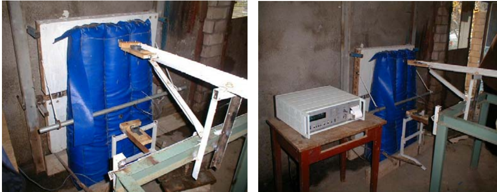
a) b) Fig.10: Reduced model using fabric envelope and filling sand.
