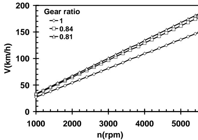
Fig. 5. Diagram of engine velocity change ( $V$ , km/h) in  $n$  (rpm) of the fourth gear with 1:1 gear ratio and 0.81 and 0.84 overdrive ratio
