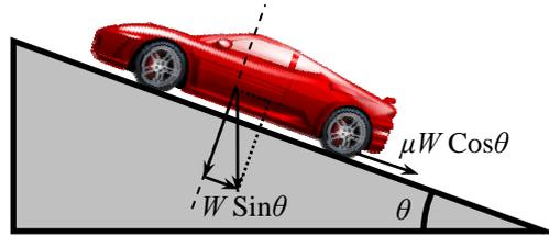
Fig. 1. Resistance force on the road slope
