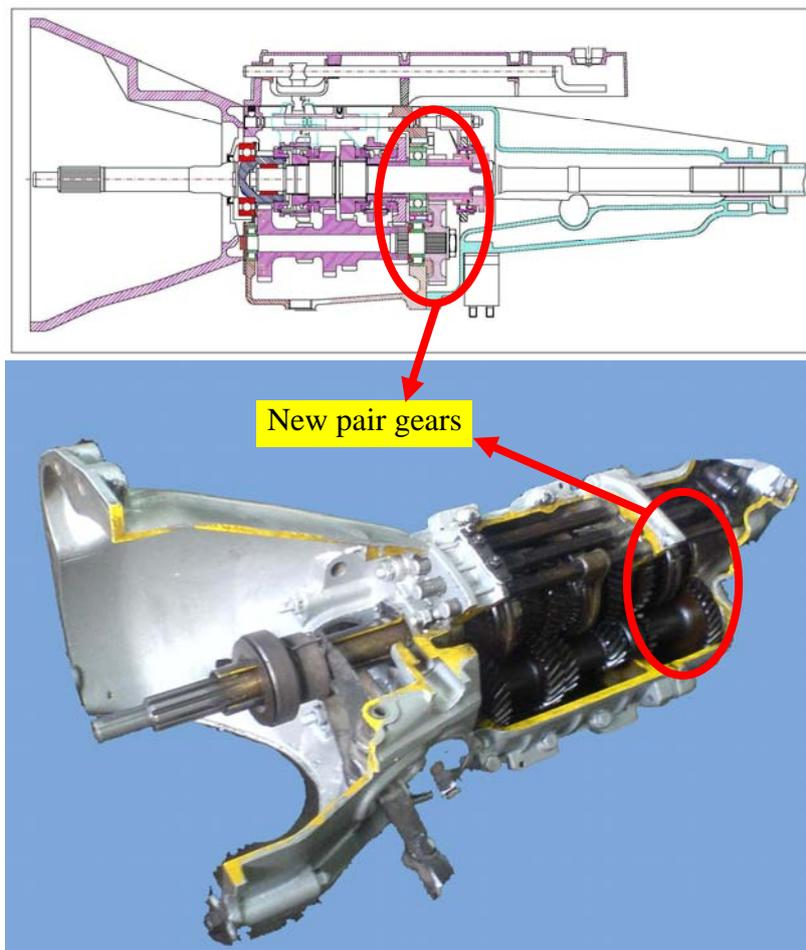
Fig. 7. Gearbox arrangement of the designed and developed models
