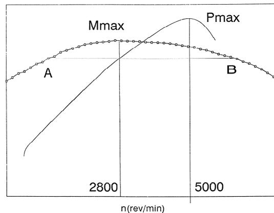
Fig. 4. The effective operation limit of the automobile
