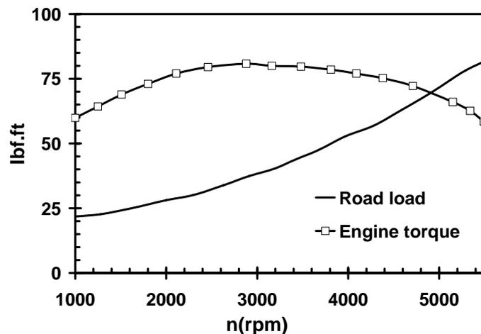
Fig. 3. Confluence curve of the road load and engine torque
