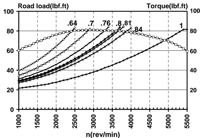
Fig. 6. Road torque diagram based on different overdrive gear ratios and the fourth gear
