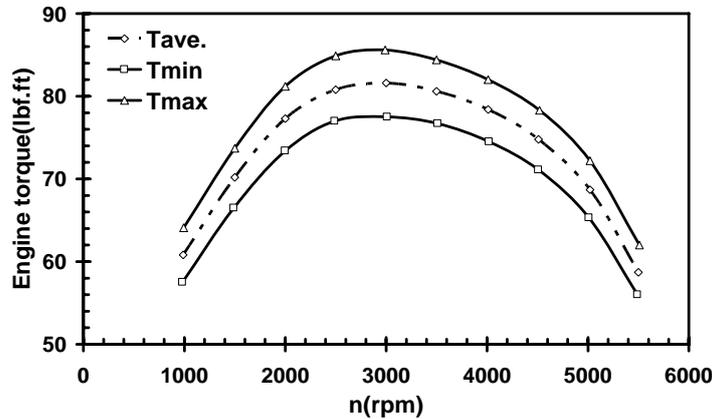
Fig. 2. Torque curve of the Roa automobile engine
