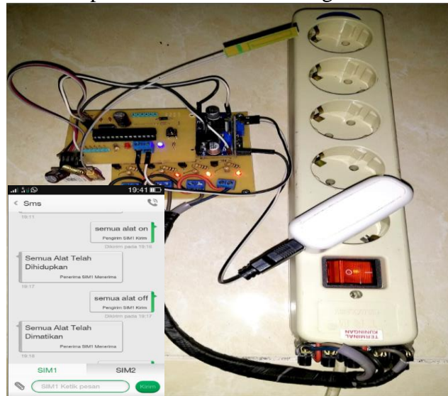
Figure 3.1 Controller on / off electronic devices.
