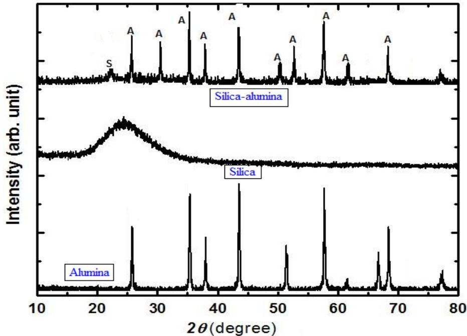
Fig. 2 XRD patterns of alumina, amorphous silica xerogel, and alumina loaded silica xerogel.
