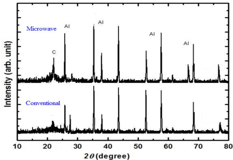
Fig. 3 X-ray diffraction graph of silica-alumina composite sintered by microwave and conventional at 1100°C
