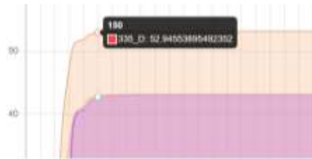
Fig. 6 The monitored state "S335" only reaches the maximum Q-value after about 150 iterations and shows that the maximum value is assigned to the "Down" action. This information can help us choose an adequate number of epochs during agent training.
