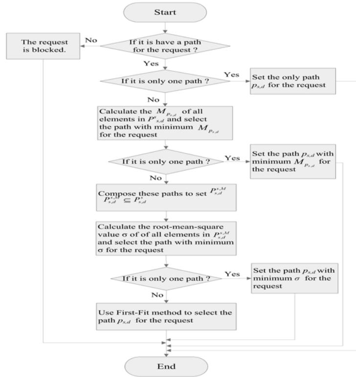
Figure 1: Flowchart of the proposed algorithm
