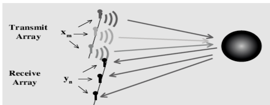
Fig. 1. System concept for m = 3 transmitters and n = 3 receivers.
