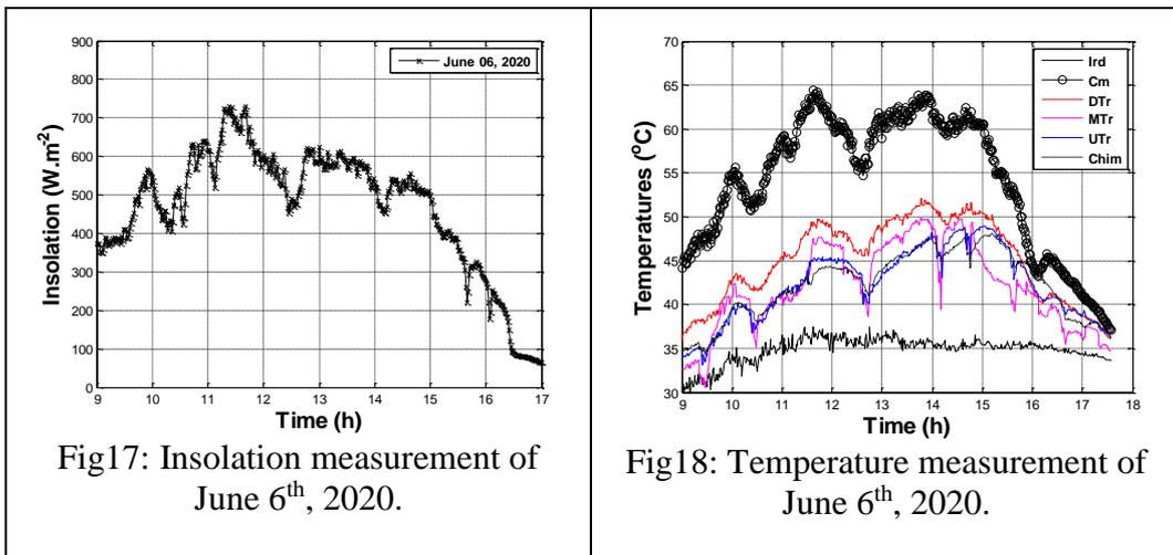
The inlet of the chamber has the highest pic of 64.4 $^{\circ}\text{C}$  at 11:38 am. Temperature pics of trays are in a gap of 47 to 52 $^{\circ}\text{C}$ .
