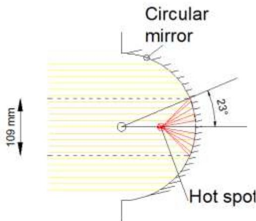
Fig3 - Parallel rays coming on the concentrator [11]
