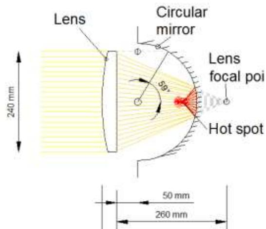
Fig4 - Deviated rays coming on the concentrator through a lens [11]
