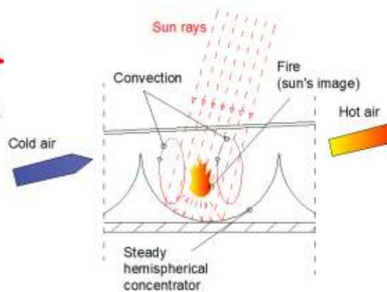
Fig2 - The hot spot principle [9].
