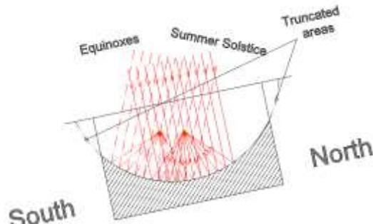
Fig6 - Truncating of the concentrator to fit the declination angle [12]
