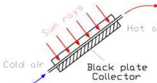
Fig1- Flat black plate collector
