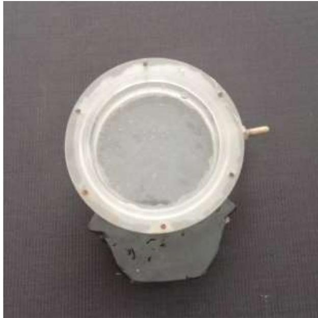
**Figure 3.** Transparent electrode with 87 mm diameter made of Hostaphan® and filled with conductive liquid (1% NaCl solution in deionized water)
