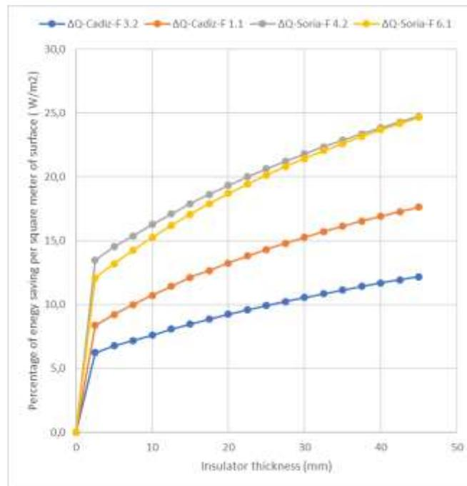
**Figure 11.** Percentage of energy saving per square metre of surface according to different thicknesses of insulation, for Soria and Cadiz according to different types of construction.
