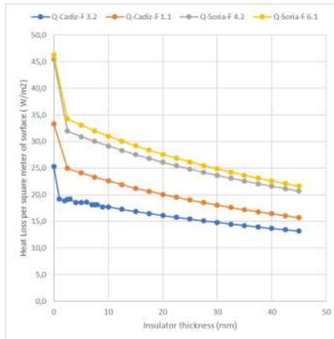
**Figure 10.** Heat loss per square metre of surface according to different thicknesses of insulation, for Soria and Cadiz according to different types of construction.
