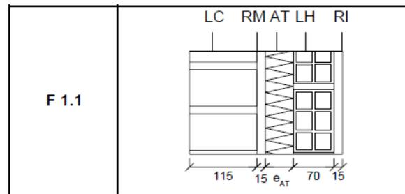
**Figure 3.** Construction detail F 1.1 according to the Technical Building Code
