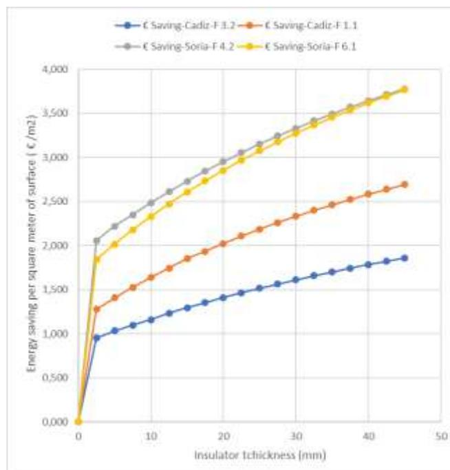
**Figure 12.** Percentage of energy saving per square metre of surface according to different thicknesses of insulation, for Soria and Cadiz according to different types of construction.
