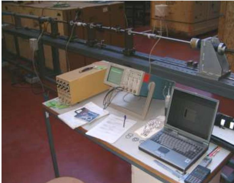
Figure 1. Equipment Hopkinson bar of damped traction of the University Carlos III of Madrid
