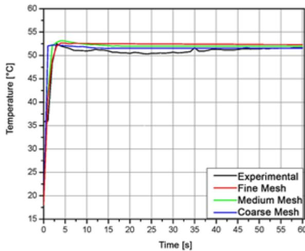
Figure 6: Behavior curves for outlet temperatures, hot water (simulated and experimental)
