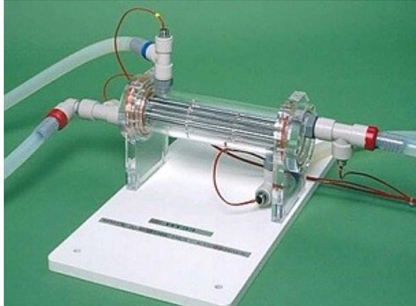
Figure 1: Shell and Tubes Exchanger
