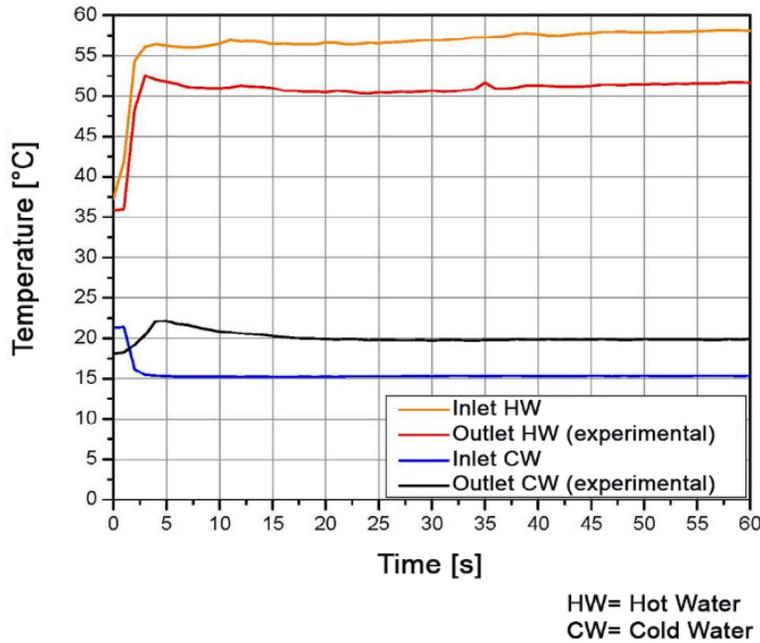
Figure 4: Experimental data of temperature vs time
