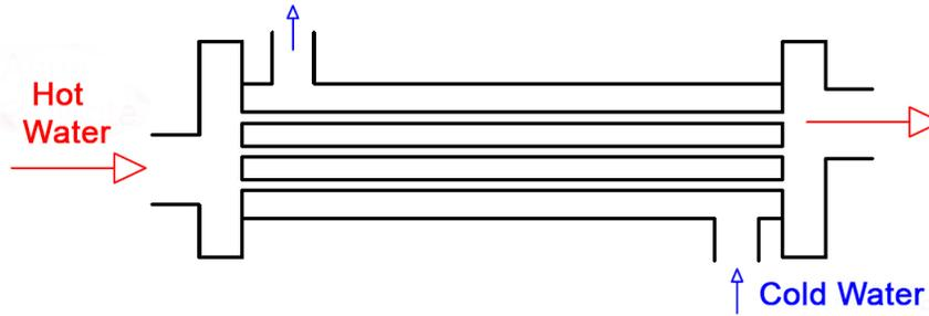
Figure 2: Direction of the flows in the exchanger (hot water through the tubes. Cold water through the shell, in a counter flow direction)
