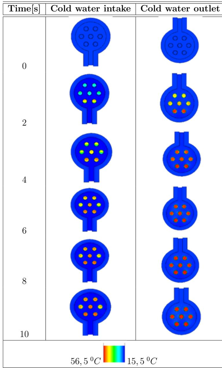
Figure 5: Simulated behavior of inlet and outlet temperatures of cold-water
