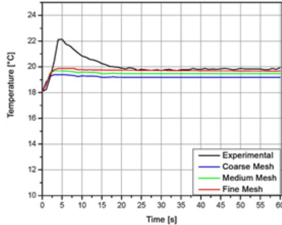
Figure 7: Behavior curves for outlet temperatures, cold water (simulated and experimental)
