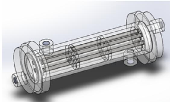
Figure 3: Three-dimensional design of the Shell and Tube Exchanger
