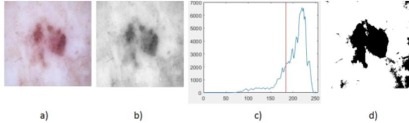
Fig 2: Digital image in a) color, b) grayscale, c) threshold by Otsu method and d) binarized image.
