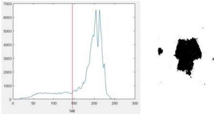
**Fig. 3:** Threshold by Otsu method.
