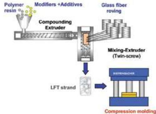
**Figure 2: Descriptive diagram of the LFT method**
