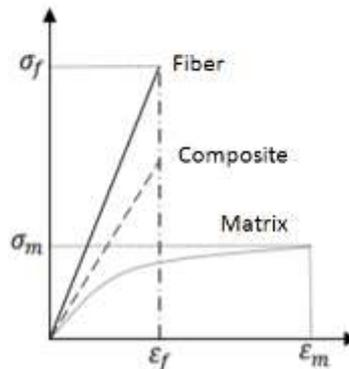
**Figure 1: Schematic curves stress / strain**
