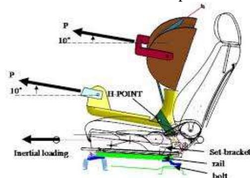
Figure 8: Belt anchor strength test
