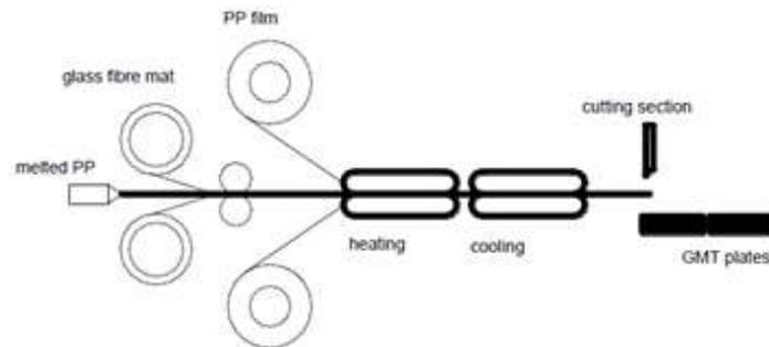
**Figure 3: Descriptive diagram of the GMT method**
