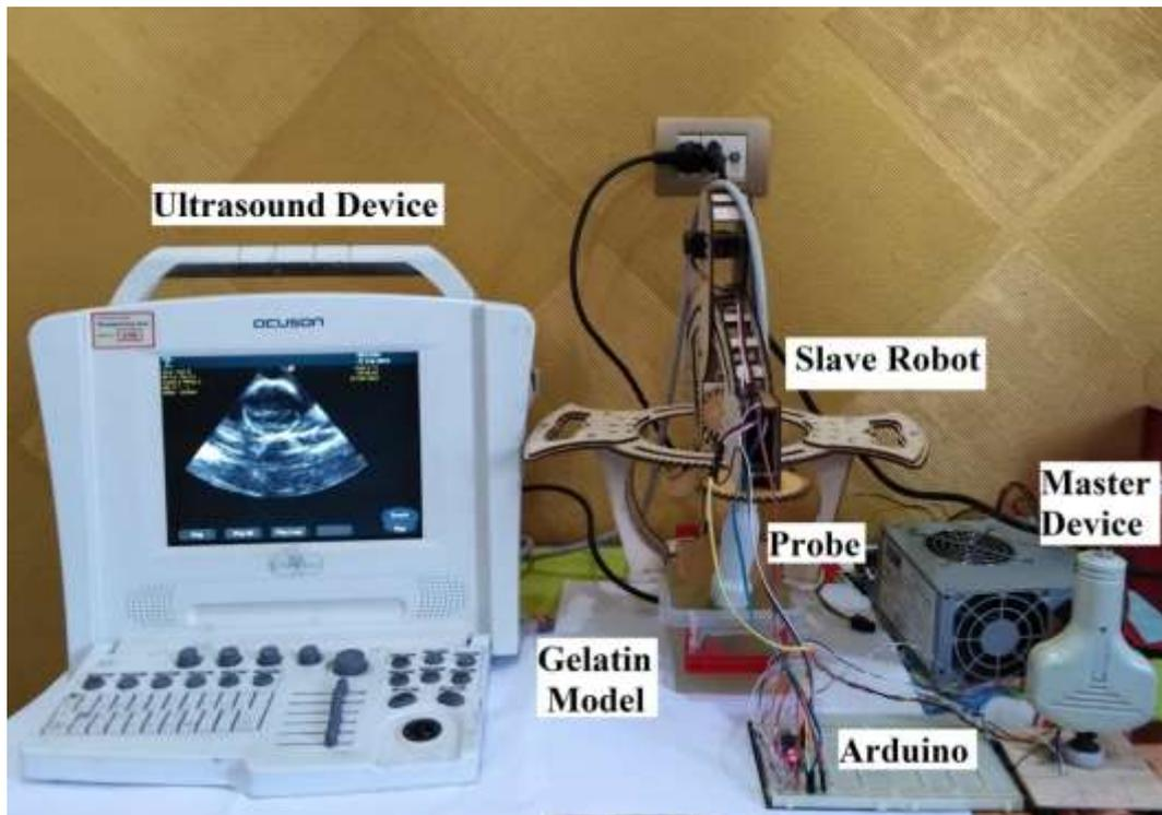
**Figure 5.** Master - Slave robotic system.
