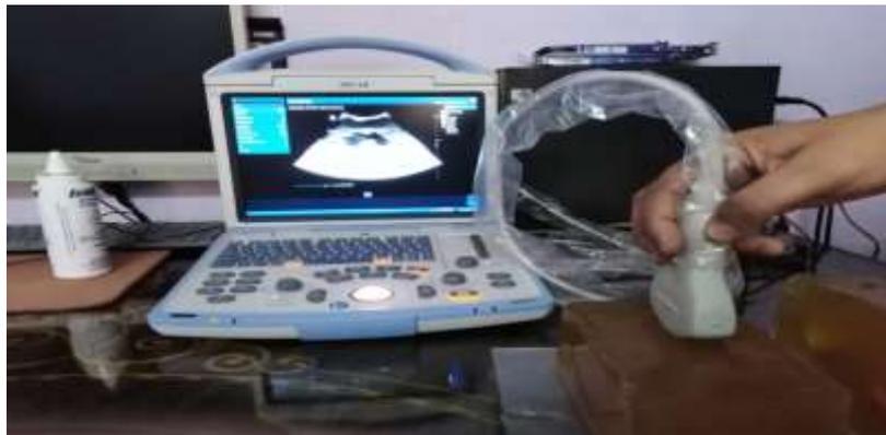
**Figure 4.** Ultrasound imaging for gelatin model
