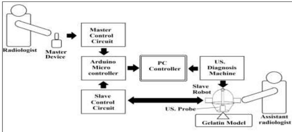
**Figure 1.** Robotic System diagram
