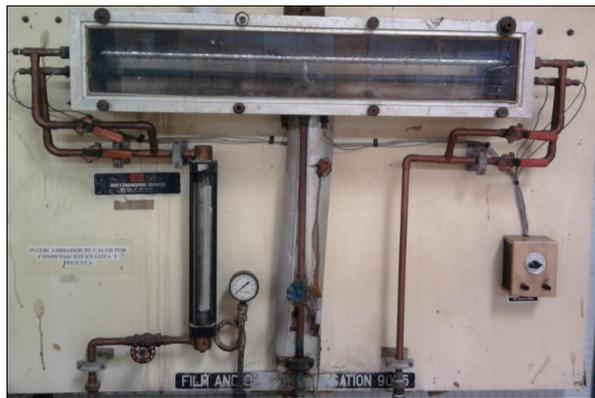
**Figure 1.** Condensation heat exchanger in drop and film
