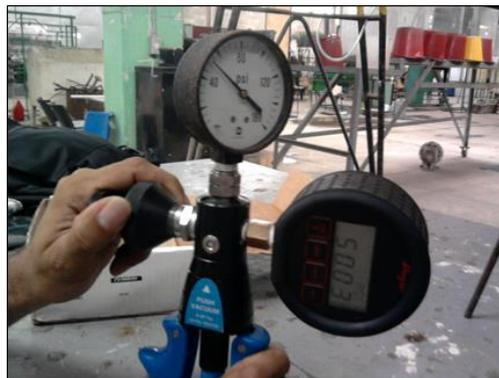
**Figure 3.** Experimental calibration of manometer
