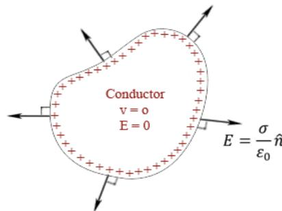
Figure 3: Conductors in electrostatic equilibrium.
