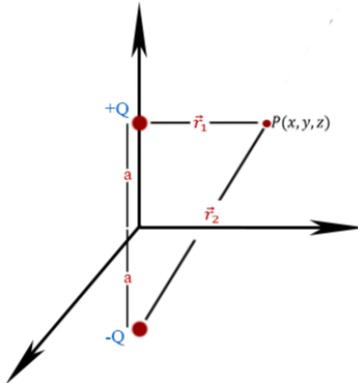
Figure 1: Electric dipole.
