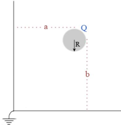
Figure 6: Conductive sphere in front of rectangular plane.
