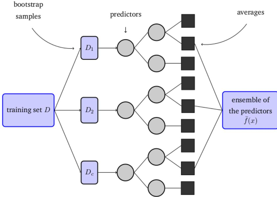
Figure 2: Operation of the bagging model, using model trees as base models.
