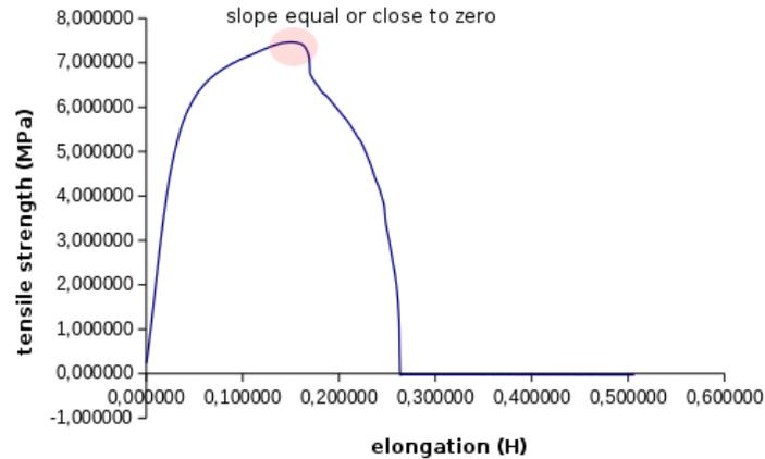
Figure 1: Material broken when the slope is less or equals to zero.
