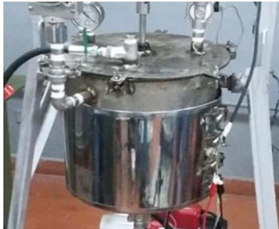
**Figure 5.** Osmodehydrator tank
