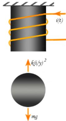
Figure 1: Magnetic levitator system.
