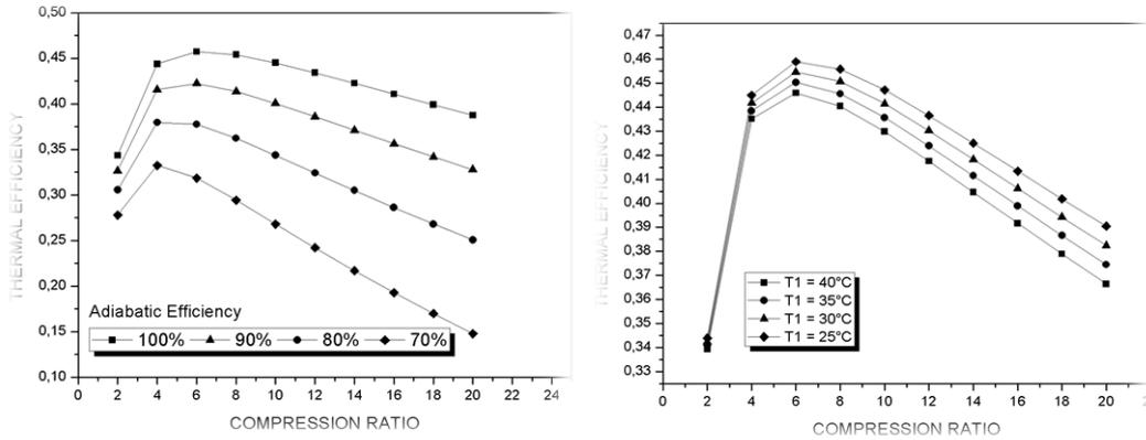
Figure 2. Results of Thermal efficiency versus compression ratio changing, a) the adiabatic efficiency, b) the inlet compressor temperature
