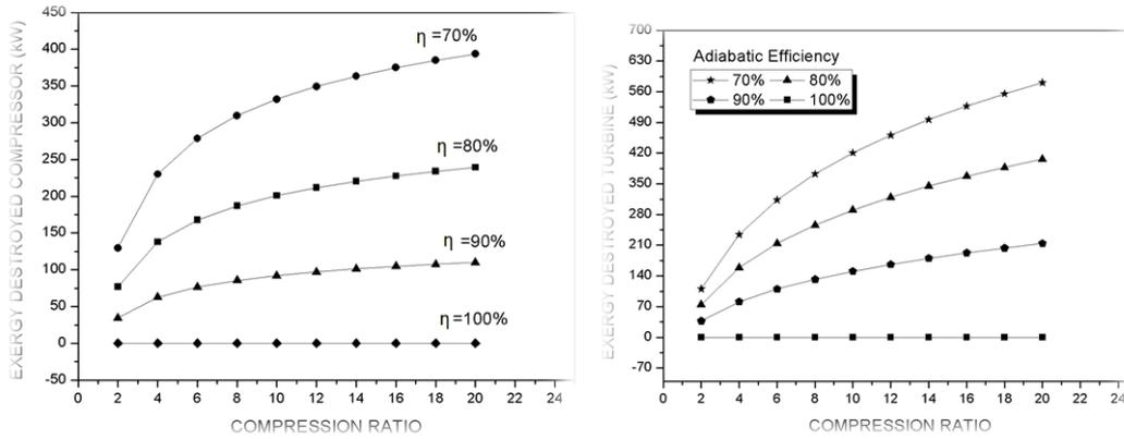
Figure 3. Exergy destroyed, a) compressor, b) Turbine
