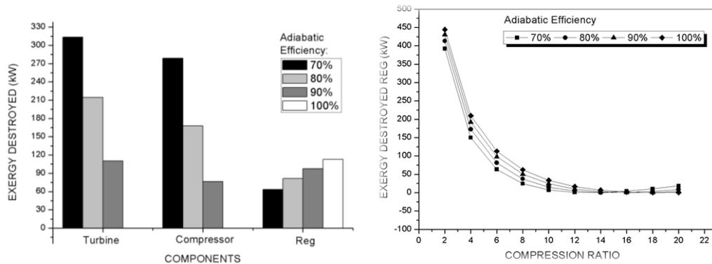
Figure 4. Destruction of exergy a) by components, b) regenerator
