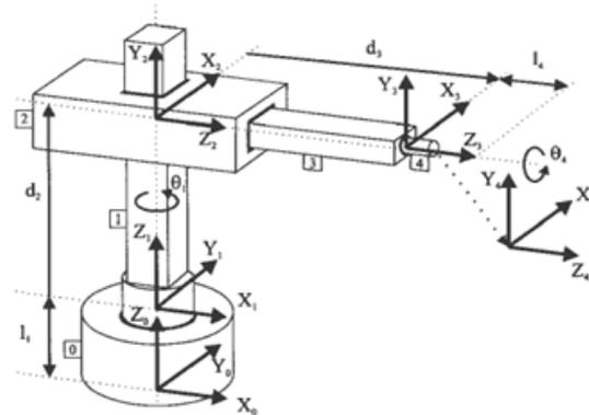
Figure 1. Robot with reference systems of the Denavit - Hartenberg method.
