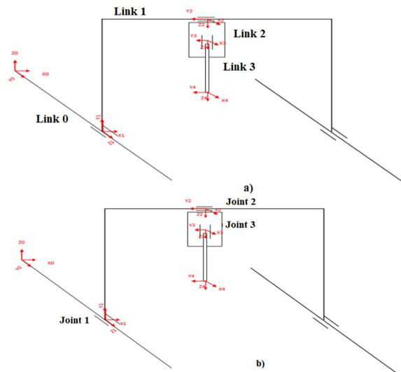
Figure 2. Cartesian table diagram with numbered, a) links, b) joints.
