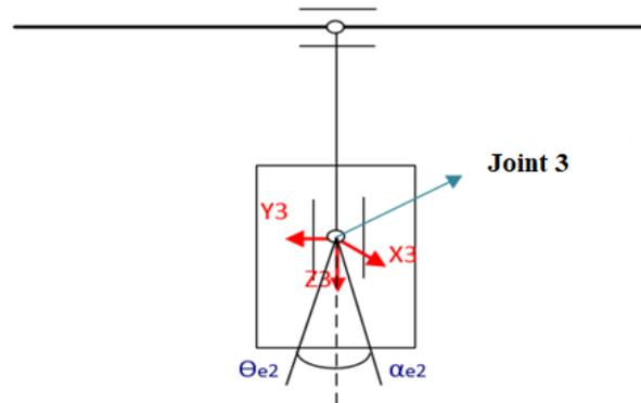
Figure 4. Perpendicularity error in articulation
