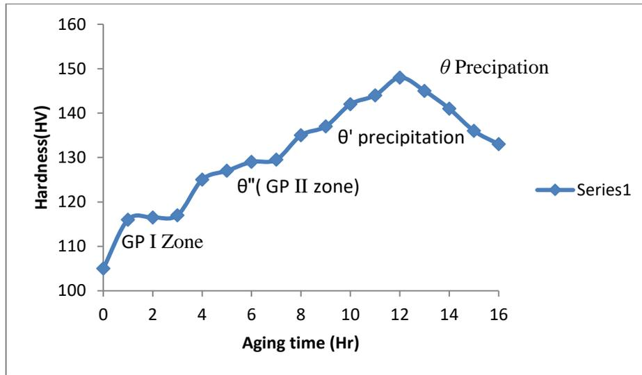
Fig. 2 Hardness Graphs with respect to aging time at 165°C for AA 2014 alloy
