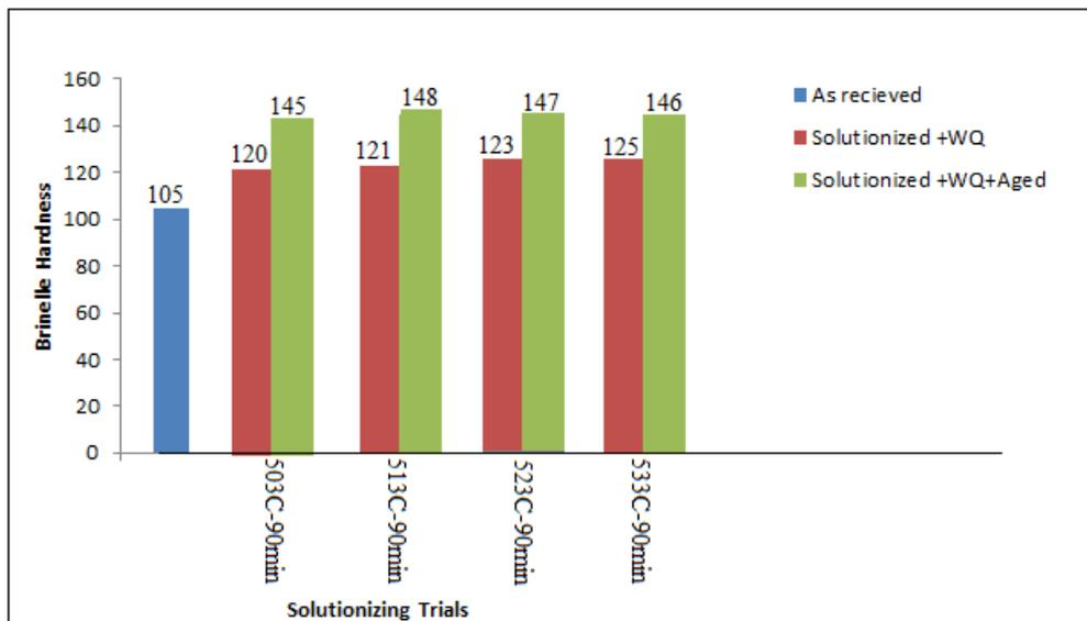
Figure 3. Effect of solutionizing treatment on hardness prior to aging at 165°C for 12 h.
