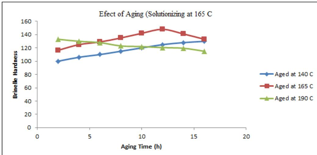
Figure (4). Comparison of aging manner of solutioned alloy aged at temperatures 140, 165, 190 °C.
