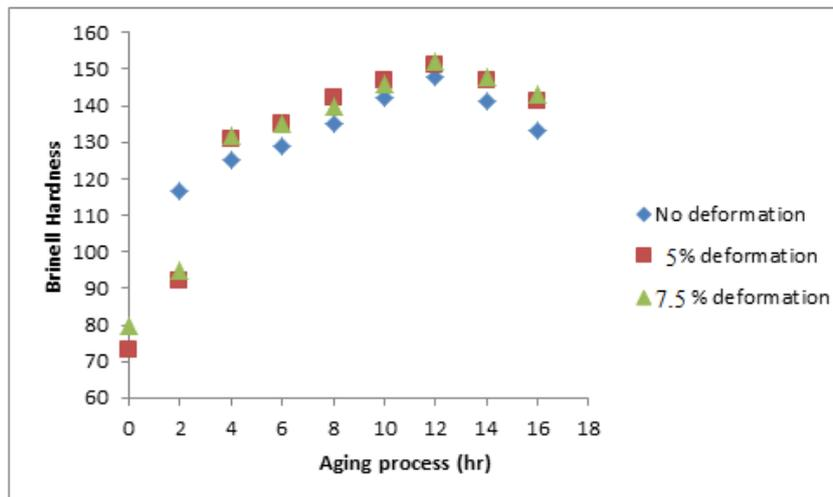
Figure (7) Influence of deformation on the hardness of AA2014 alloy
