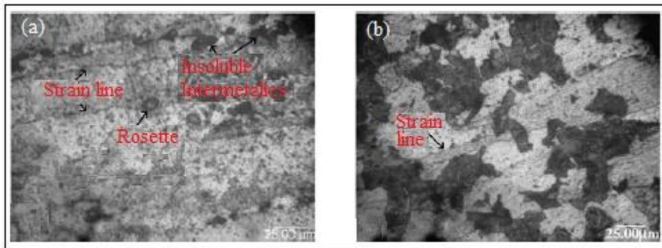
Figure (5) optical micrograph of 2014 aluminum (a) at solution treated (b) after aging for 8 hr
