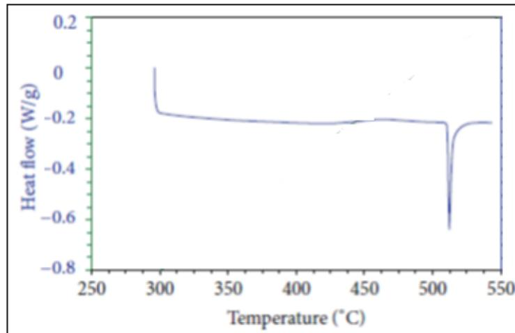
Figure (1) DSC curve for AA2014 alloy
