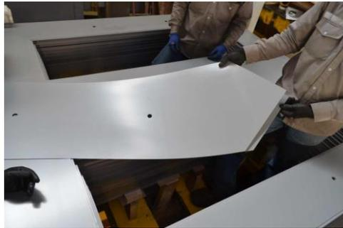
Figure 1. Ferromagnetic core lamination.
