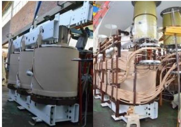
Figure 3. Transformer active part
