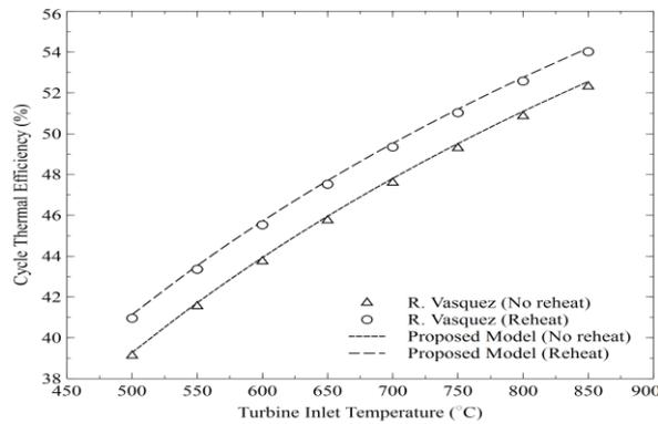
Figure 3. Validation of the proposed model with and without reheating, according to reference. R. Vasquez [4]. Input data are given in Table 1.
