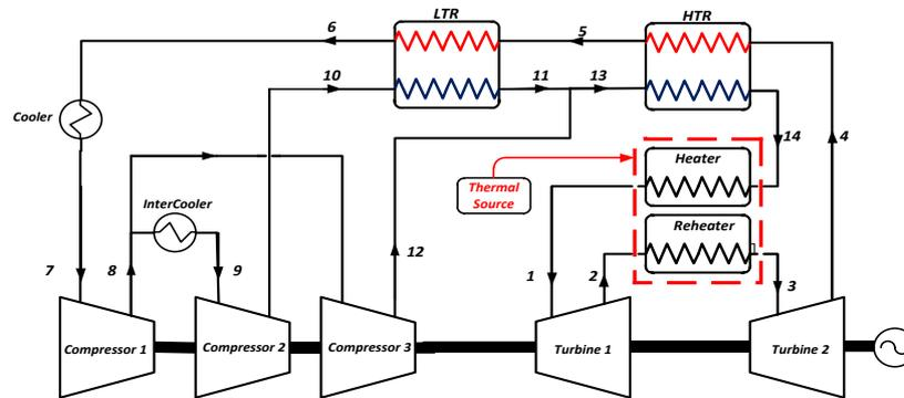
Figure 1. Supercritical  $s - CO_2$  PC Brayton Cycle Layout. Adapted from [4]
