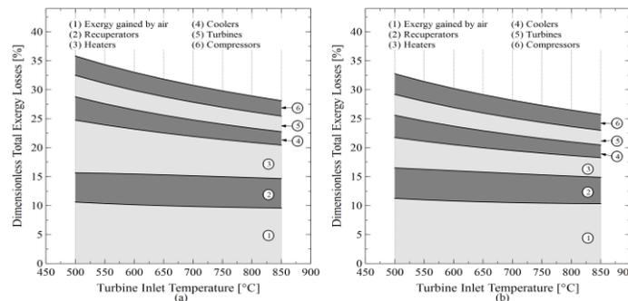
Figure 4. Dimensionless exergy losses by component for Partial Cooling S- $CO_2$  Brayton cycle. (a) without reheat, (b) with reheat.
