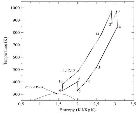
Figure 2. Temperature-Entropy diagram for Supercritical ( $s - CO_2$ ) Partial Cooling Brayton Cycle Layout with reheat.
