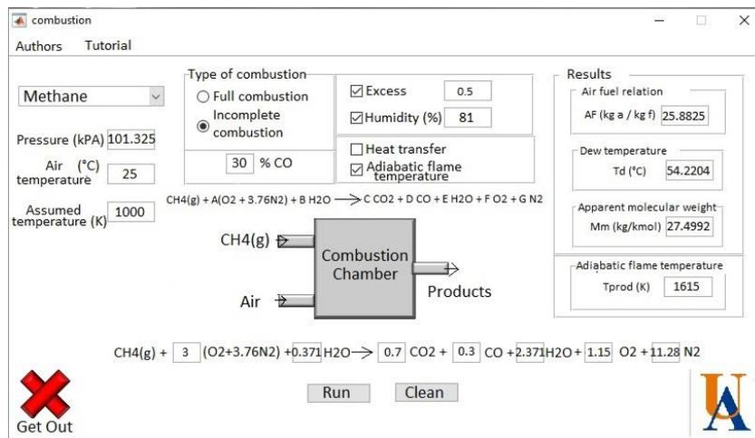
Figure 1. View of the CombustionUA software.
