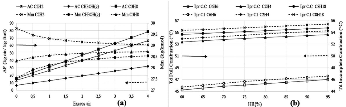
Figure 2. a) Results of the Excess Air Analysis, b) Results of the Relative Humidity Analysis.
