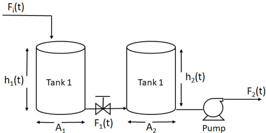
Figure 1. Diagram of system of tanks in interacting mode
