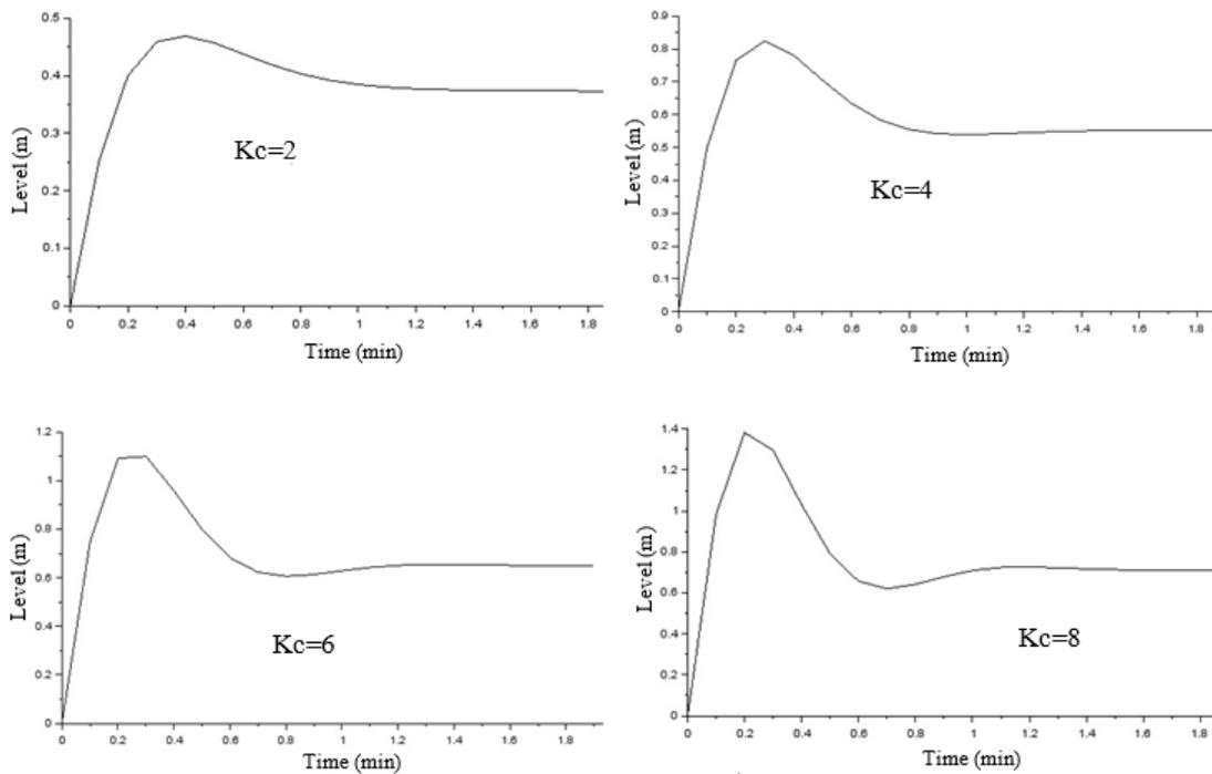
Figure 3. Simulation of feedback level control of tank 1 in interacting mode. Proportional feedback with a)  $K_c=2$ , b)  $K_c=4$ , c)  $K_c=6$  and d)  $K_c=8$
