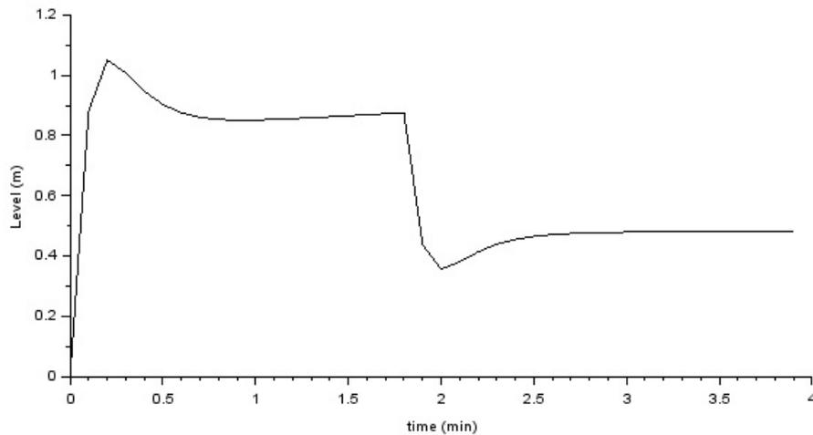
Figure 4. Simulation of PID feedback level control of tank 1 in interacting mode with step changes in set point of tank 1 level and disturbance in the pump flow.
