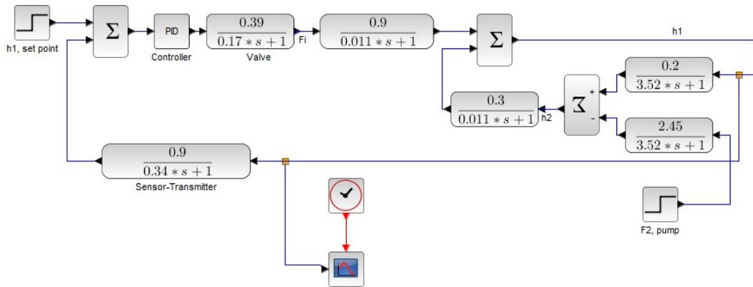
Figure 2. Diagram of blocks of a system of tanks in mode interacting for simulation
