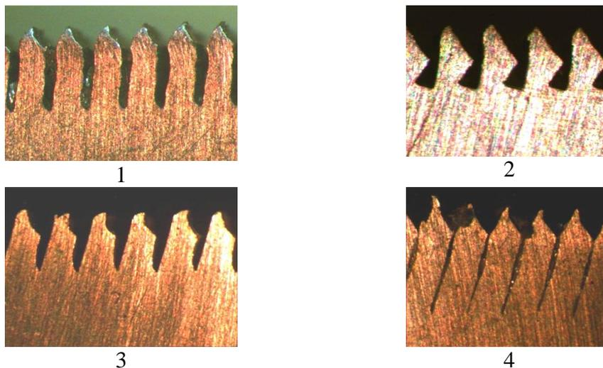
Figure 3. The types of microstructured pipe (Type №1, №2, №3, №4)
