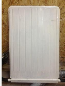
Figure 8. Prototype of radiator based on independent evaporate circuit
