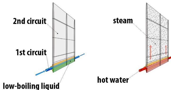
Figure 1. The principle of the independent evaporate circuit in the radiator
