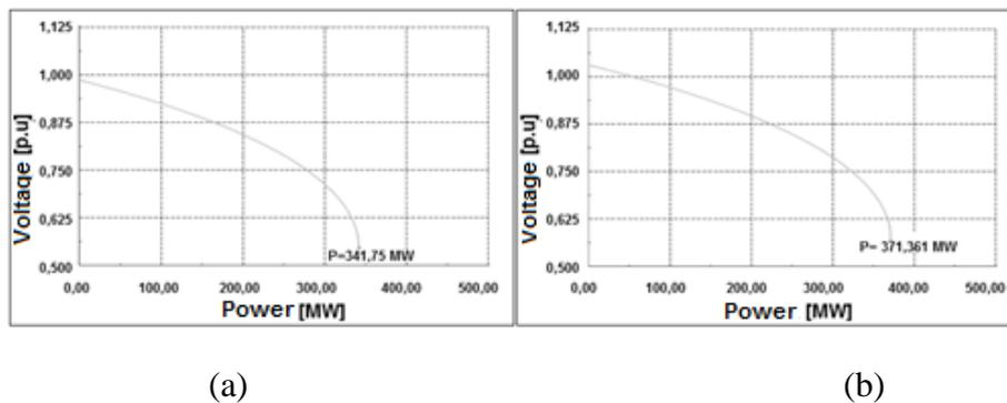
**Figure 10.** PV curves on industrial node 7, scenario 5. (a) Before integration. (b) After integration
