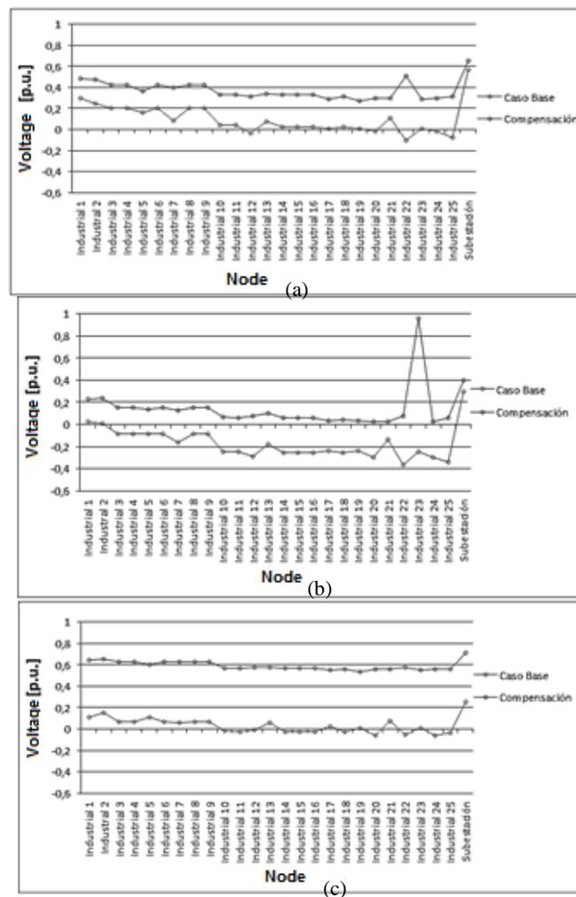
**Figure 9.** Voltage index per node a) Scenario one. (b) Scenario three. (c) Scenario five
