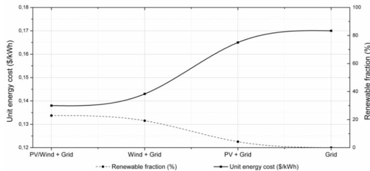
**Figure 6.** Unitary energy cost and Renewable fraction comparative
