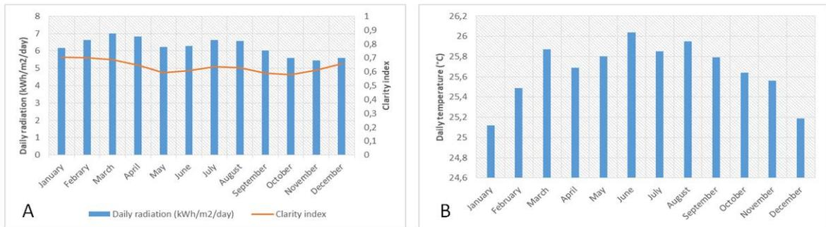
**Figure 2.** Energy source: a) RHG Solar resource, b) daily temperature.
