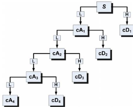
Figure 5. Wavelet decomposition tree [14]
