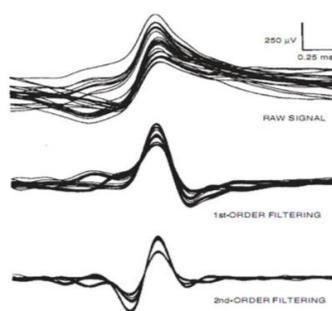
Figure 4. Effects of bandpass filter as order increases [11].
