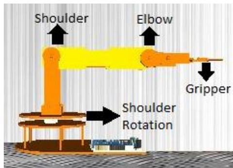
Figure 12. Manipulator joints.
