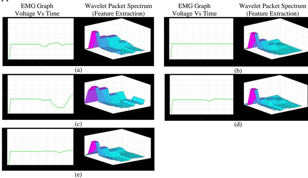
Figure 13. Behavior of the input signal and feature map for each gesture: (a) Fist, (b) Relax, (c) Wave\_In, (d) Gun and (e) Close\_Fingers.
