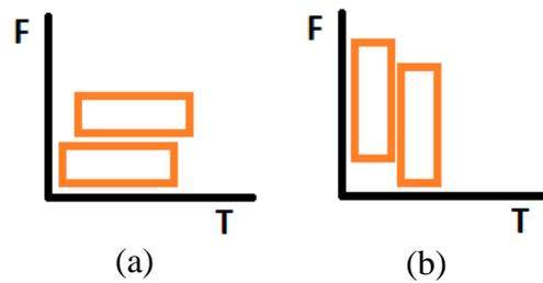
Figure 7. (a) Time Domain Filter. (b) Frequency Domain Filter.
