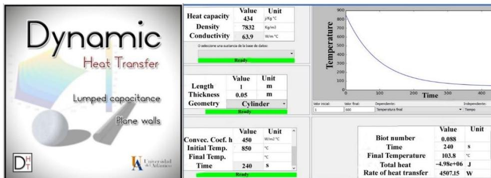
Figure 1. Interface software DynamicHT Lumped Capacitance
