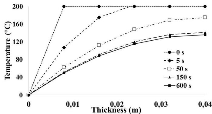
Figure 3. Temperature gradients within the plane wall
