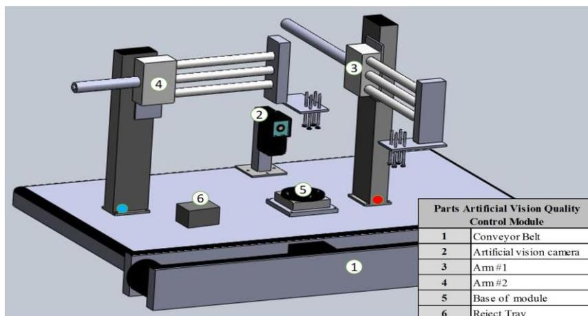
Figure 3: Components of station 6 (Station FMS-210).
