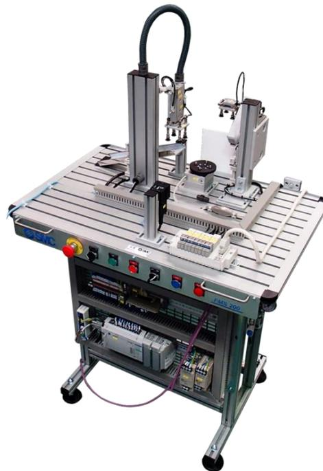
Figure 1: FMS-210 artificial vision quality control station [10]
