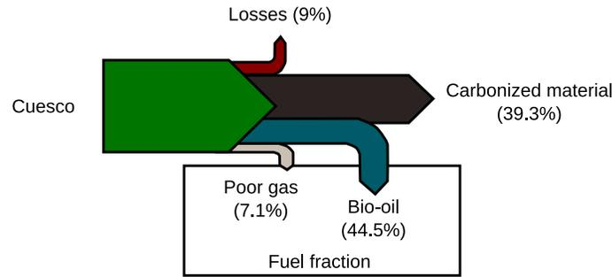
Figure 2: Sankey diagram of material proportion (carbonization furnace) [4]
